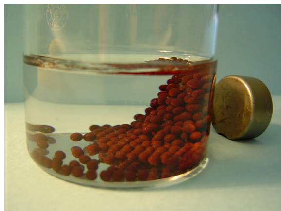
Fig. 2. Photograph of magnetic alginate beads attracted by a magnet.
